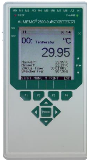
Figure 2. ALMEMO 2890-9 type data logger
