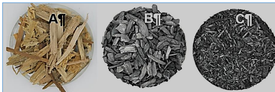
Figure 1. Wood waste (A), processed into biochar (B) and biochar processed from short-blade grass (C).
