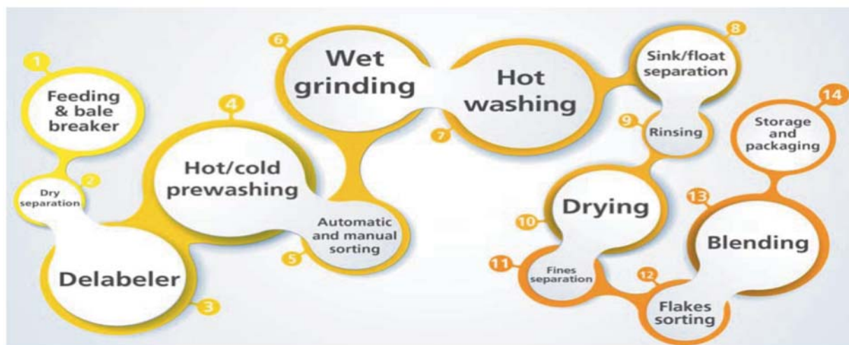
Figure 1. PET plastic recycling steps
