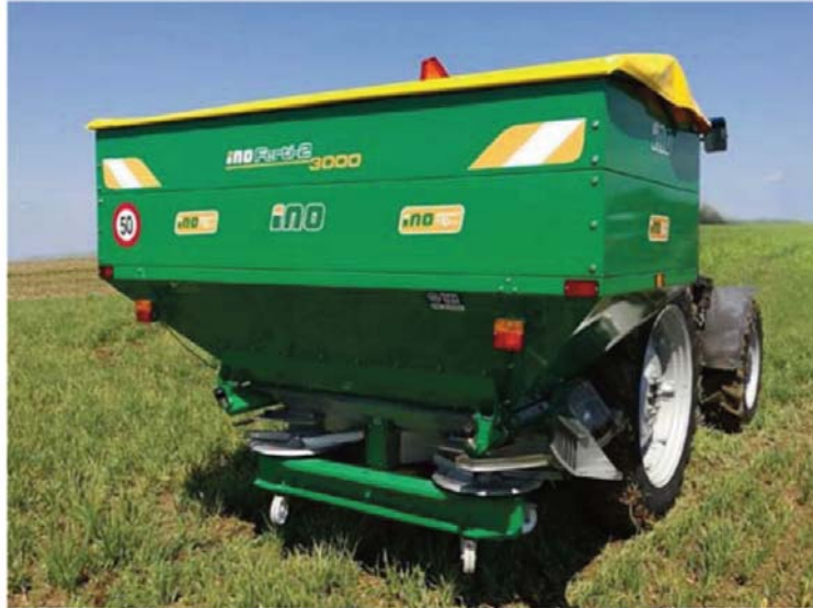
Figure 1. Double-disc mounted fertiliser spreader FERTI-2 (Source: INO)
