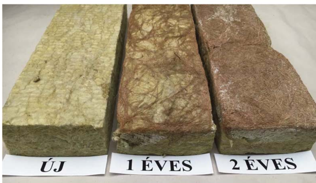
Figure 3. Rockwool slabs (upside down) from the experiment: before usage (left), after the first growing season (center), after two growing seasons (right)
